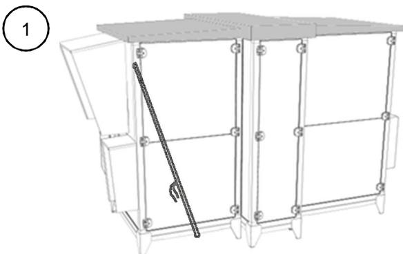
1. Securing eyelet must be tied using a tying mechanism (rope) -> the door is secured in case of wind
